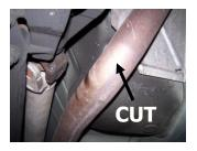
**3.** Then cut over axle tail pipe before axle and remove.
